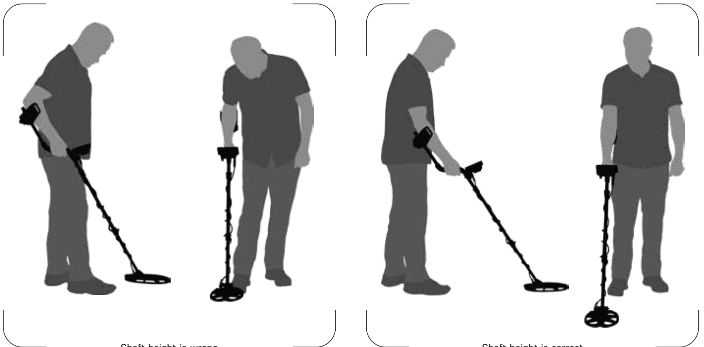
Shaft height is wrong
