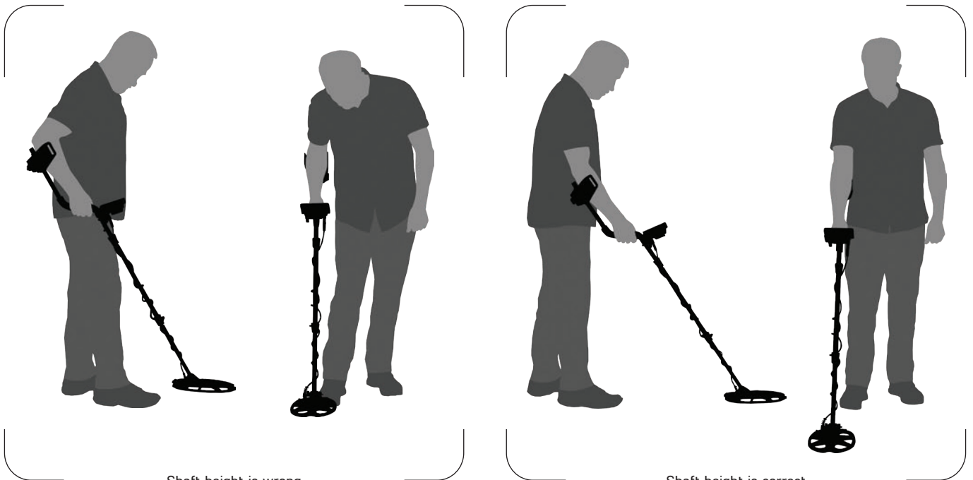
Shaft height is wrong
