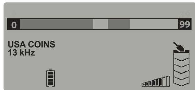
USA Coins Mode as it appears on a VX5 with single-tier Target ID scale or on VX7 and VX9 when operating in a Single Frequency.
