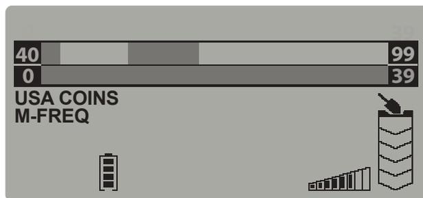
USA Coins Mode as it appears on a VX7 with two-tier Target ID scales in Multi-Frequency operation.
