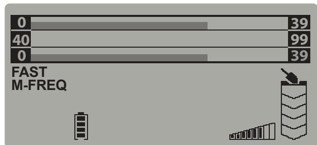
Fast Mode on VX9 model, showing suppressed response on common ferrous targets. This three-tier Target ID scale becomes a single scale while in a Single Frequency.
