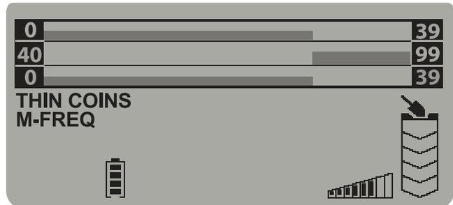
Thin Coins Mode on VX9 model, showing suppressed response on common ferrous targets and high conductors. This three-tier Target ID scale becomes a single scale while operating in a Single Frequency.
