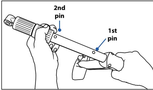
Loosen upper camlock and extend stem until pin locks into first pin position. Hand-tighten upper camlock. (Note: second pin position can be used to extend stem length.)
