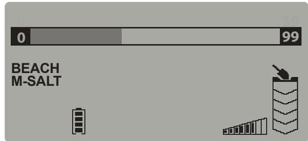
Beach Mode on VX7 and VX9 models, displaying a single-tier Target ID scale and operating in Multi-Salt frequency.
