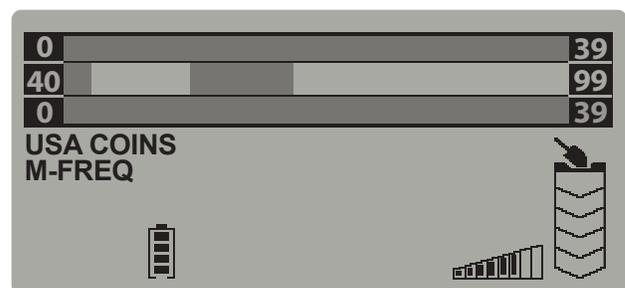
USA Coins Mode as it appears on a VX9 with three-tier Target ID scales while operating in Multi-Frequency.
