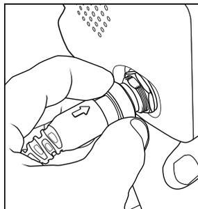
◀ Wrap cable around stem and attach.
