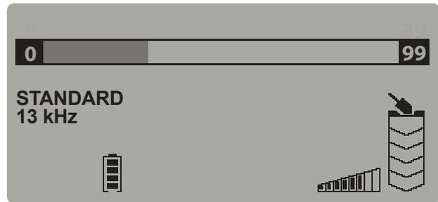
Standard Mode as it appears on a VX5 with single-tier Target ID scale or on VX7 and VX9 when operating in a Single Frequency.
