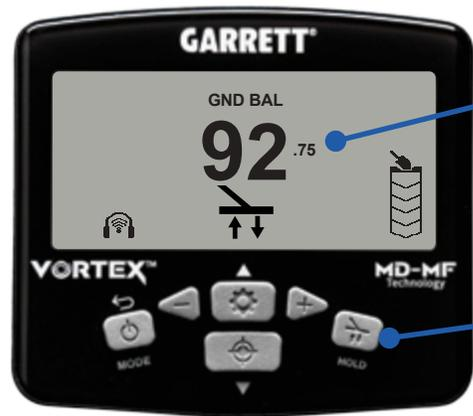
Ground Balance reading of 92.75 indicates highly ferrous soil content.
