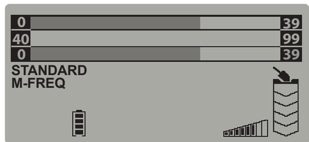
Standard Mode as it appears on a VX9 with three-tier Target ID scales while operating in Multi-Frequency.
