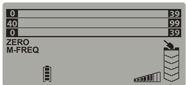
Zero Mode as it appears on a VX9 with three-tier Target ID scales while operating in Multi-Frequency.
