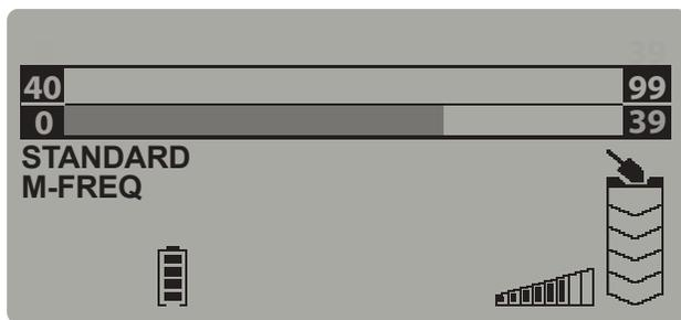
Standard Mode as it appears on a VX7 with two-tier Target ID scales in Multi-Frequency operation.
