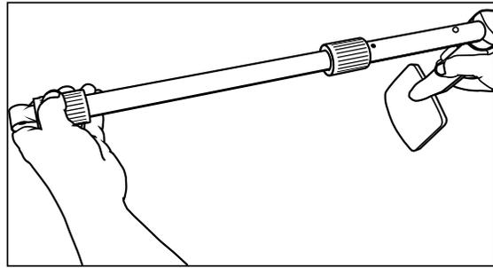
Loosen lower camlock and extend stem to desired operating length. Hand-tighten the camlock. (Note: do not tighten the camlocks without a stem inserted into them.)
