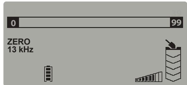
Zero Mode as it appears on a VX5 with single-tier Target ID scale or on VX7 and VX9 when operating in a Single Frequency.
