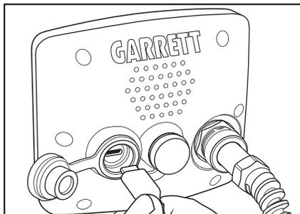
◀ Insert USB-C to charge unit. Use 10W (2A) or greater power source for fastest charging time. Lower wattage source will take longer.
