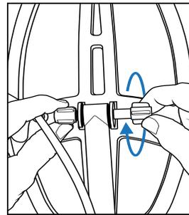
◀ Insert rubber washers, connect searchcoil to the stem as shown, and hand-tighten the wing nut.
