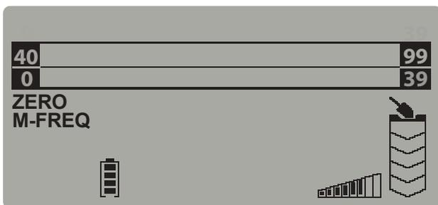
Zero Mode as it appears on a VX7 with two-tier Target ID scales in Multi-Frequency operation.
