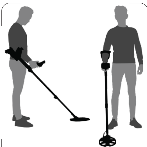
Shaft height is correct
