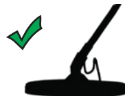
Correct search coil angle
