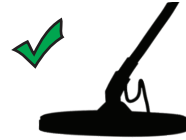
Correct search coil angle
